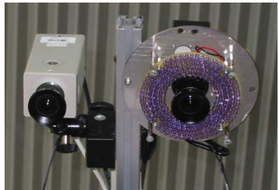
Figure 4. The camera used for passengers counting (right), with its infrared lighting system (221 LED's). The camera on the left is used for reference manual counting.
