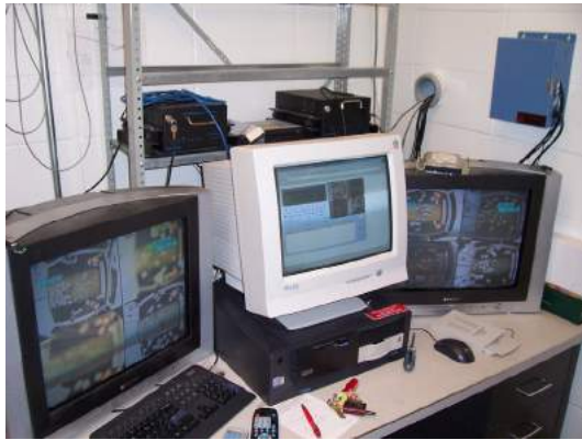
Figure 1. Sentry SMD-04 4 Channel Embedded Mobile Digital Video Recorder being used for acquiring video files for behavioural tracking with EthoVision software. Two 250Gb hard drives are situated at the back to store the video files which can be viewed on one of two monitors. The computer monitor in the center is remotely displaying the arenas over the internet.
