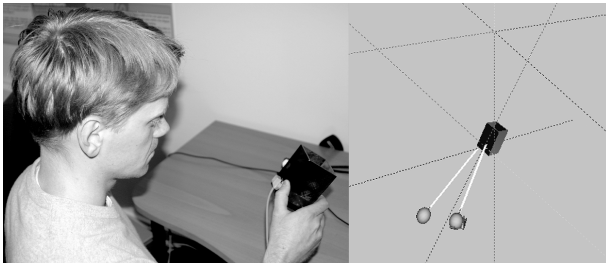
Figure 2 Measurement setup and the virtual model showing the eyes, their gaze vectors and resulting gaze points on the surface of the object.
