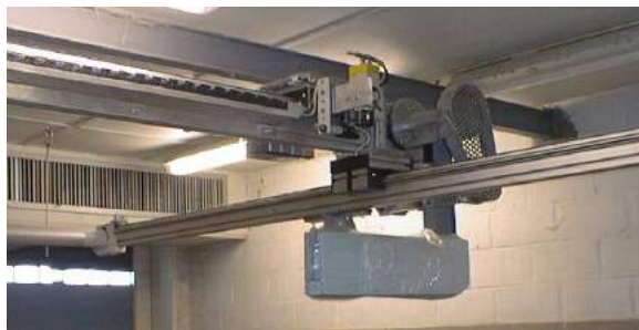
Figure 2. Digital camera installed on an automatically controlled rail system.
