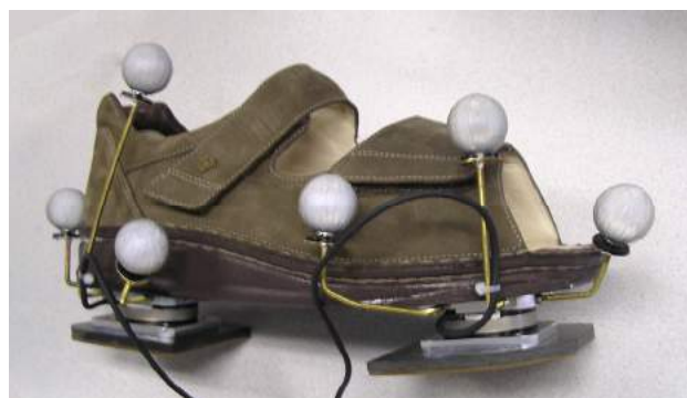
Figure 1. Shoe instrumented with two 6-axis force sensors. Reflexive markers are added for position analysis using the VICON optokinetic system (not evaluated in this paper).
