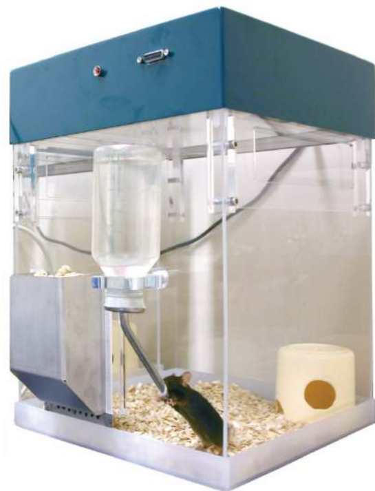
Figure 1. The PhenoTyper ® home cage is used for high throughput phenotyping. In a battery of these cages single mice are housed for a week, subjected to a large number of behavioral tests and data is acquired using an overhead camera and video tracking software.
