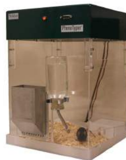
Figure 1. Single cage with top unit of the PhenoLab® system for automated home cage observations. Each cage contains a fixed water bottle, feeding station and shelter.
