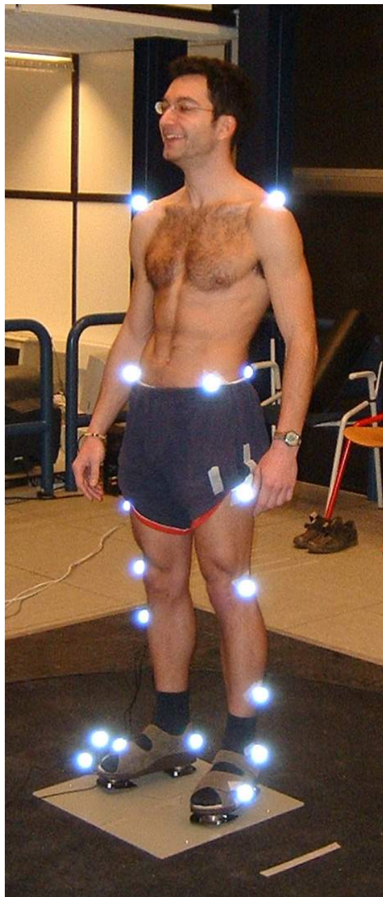
Figure 2. Subject standing on instrumented shoes. Only the right shoe is instrumented with two 6 DOF forces, the left shoe contains two dummies.
