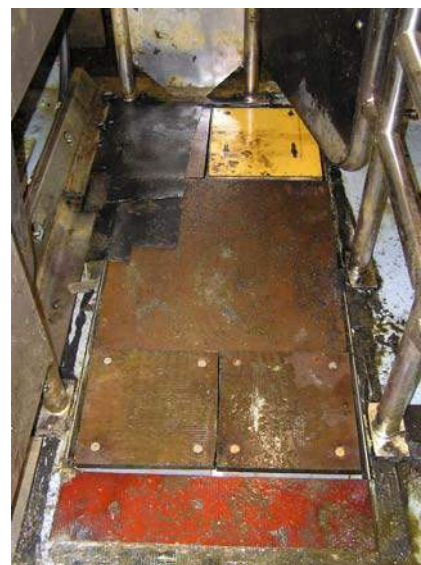
Figure 2. The plywood plates on top of the balances as they are positioned on the floor of the milking robot
