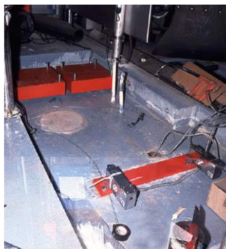
Figure 1. The strain gauges on the floor of the milking robot.
