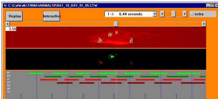
Figure 1. A rat walking, from right to left, through the CatWalk corridor. Top panel: Snapshot of the rat in the corridor where false colours represent the different intensities of the signal (red=low, blue=high). Middle panel: Track of footprints from one passage (right paws in green, left paws in red; front paws light, hind paws dark colour). Bottom panel: The time of floor-contact by the different paws. Blue dotted lines indicate seconds, and the white dotted line the snapshot in the top panel
