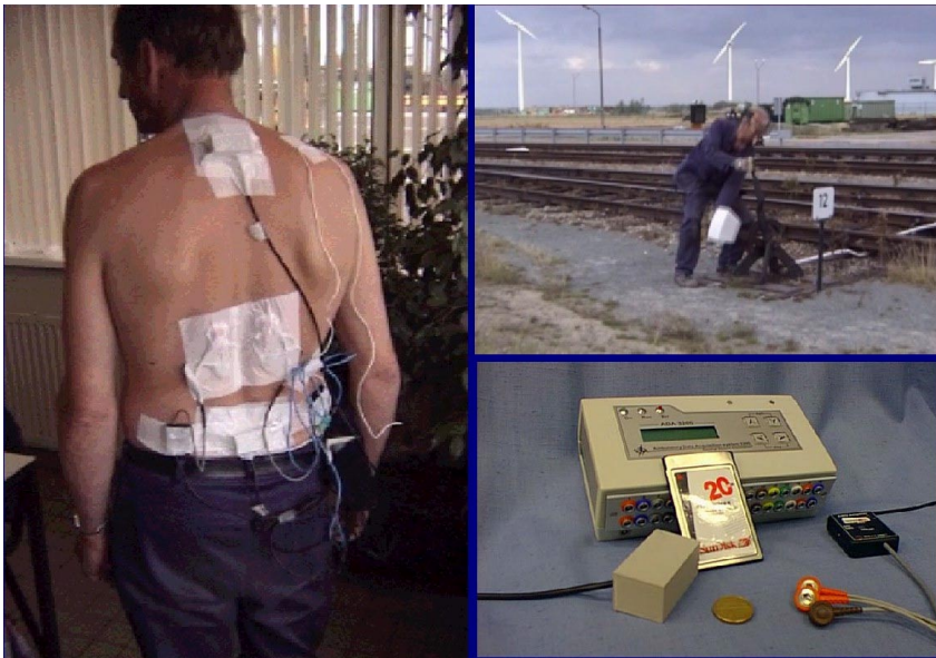
Figure 1. Physical setup of an AMBER monitoring session. A. Inertial sensors are placed on the skin of the back above vertebrae L3 and T10; surface EMG sensors are placed on the skin above the erector trunci at levels L3 and T10, 3 cm left and right of the middle axis. The data acquisition module is placed at the waist (right side). B. A railway employee with an AMBER system mounted performing his job unhindered. C. The AMBER recording hardware.
