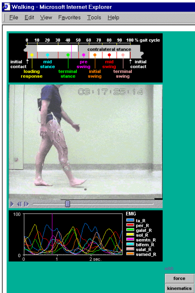
Figure 1. The graphical user interface of the HTML viewer as it appears in a web browser. The time lines in the figures with kinesiological data are synchronized with the video player. Video time can be set by mouse clicks in the figures.
