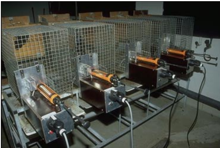
Figure 2. Rear view of four chambers. showing the feeders.
