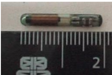
Figure 2. A 19-mm transponder.
