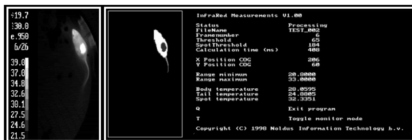
Figure 1. Left: sample of a thermographic recording of a rat. Grey values correspond to temperatures (see index bar on the left). Note the shaven spot (light) on the rat's back. Right: Image after analysis: computer discriminates tail (24.00 °C) and shaven spot (32.34 °C) from the rest of the body (20.06 °C).
