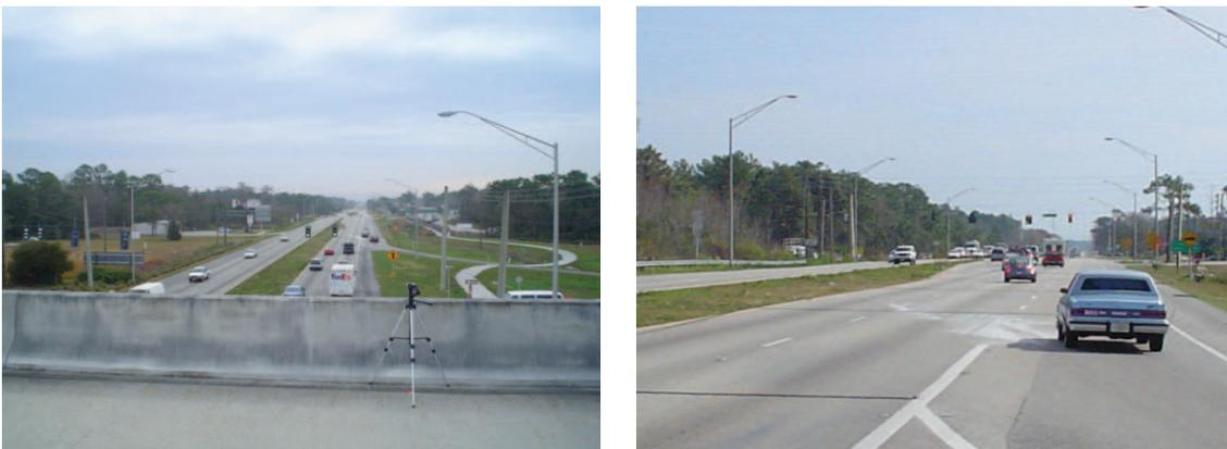
Figure 3. Video camera positioned on the bridge and road tubes placed every 100 feet along the arterial.
