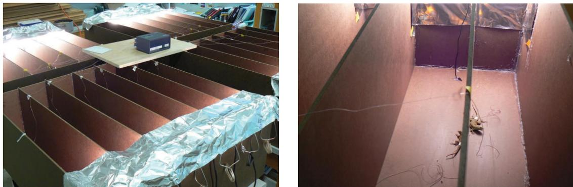
Figure 1. Experimental set up for recording T<sub>b</sub> in laboratory using Eltek squirrel automated data logger. Up to 24 lizards can be recorded simultaneously in parallel tracks which are illuminated using lamps to create thermal gradients.
