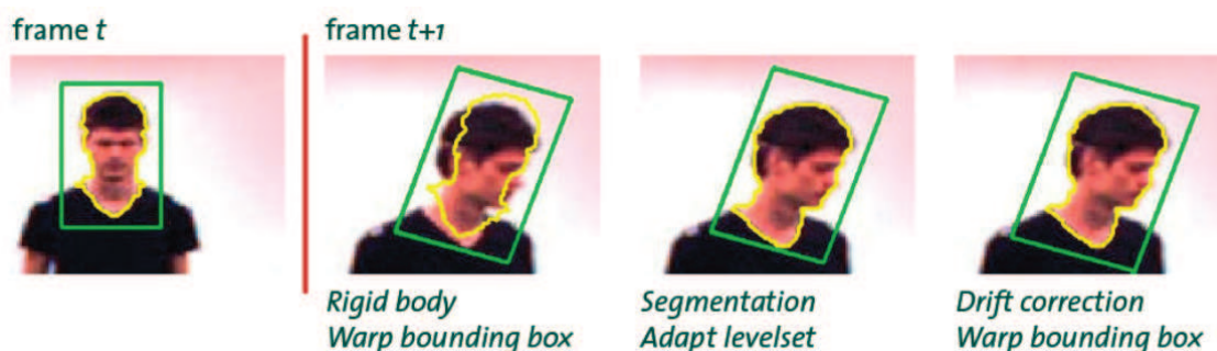
Figure 1. Principle of level set based contour tracking: the bounding box (green) including the initial segmentation (yellow) are given in time step t . In the next time step t+1 , the rigid body tracking, the re-segmentation and the drift correction step are given.
