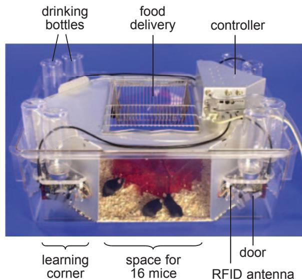
Figure 1. The IntelliCage apparatus.
